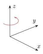
with x corresponding to real values, y imaginary values, and z time. In this frame a positive rotation is defined as counter-clockwise looking down the time axis (shown in red). The spectral data points are ordered in sequence of increasing time.
